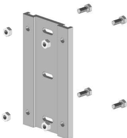
**PS135M250 + DIN933M10x25mm + DIN934M10 :**
